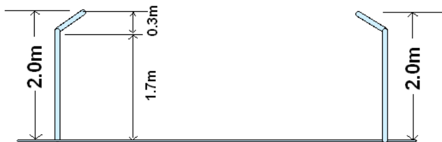
Fig. 9: Reflective Noise Barrier of height 2.0 meter
